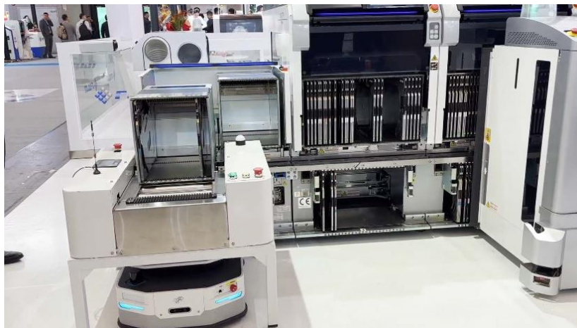
At productronica China 2025, Standard Robots' Oasis-300E AMR was used to transport part supply magazines to Fuji's NXTR A model pick and place machine
