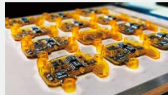
Sample prototypes of a power circuit board for a custom robot
