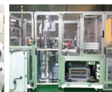
Automation of the production process (automatic machine for NXTR bed underside roller assemblies)
