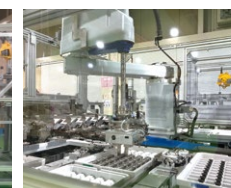
Automation of the production process (automatic machine for NXTR bed underside roller assemblies)
