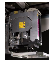
Placement of a large, heavy component for an AI server
